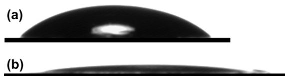
Fig. 6. Photograph of the (a) water droplet and (b) octadecane droplet on the film of system A.
